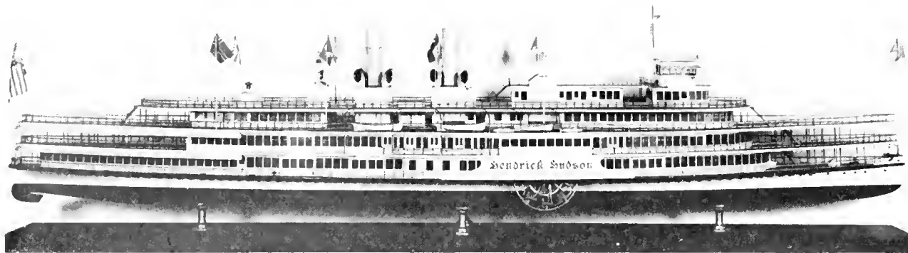
THE STILL SIDE-WHEEL HUDSON RIVER STEAMER Hendrick Hudson was built by the Marvel Shipbuilding Company, Newburgh, New York, in 1906. Licensed to carry 5,500 persons, she ran for many years between New York City and Albany. Rigged model USNM 309408. (Smithsonian photo 47162.)
